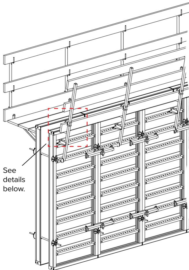
The Toe Board Retainer, marked with red paint, is attached to the Counter Post in the following way:
