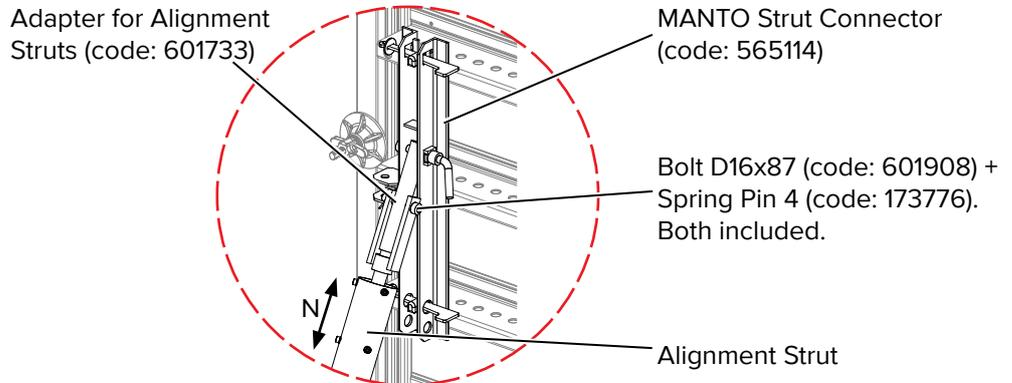
To connect the struts to **horizontal panels** insert the Adapter for Alignment Struts into the strut and secure using the an additional Bolt D16x87 and the Spring Pin 4. Attach the MANTO Strut Connector to the panel ribs using the integrated wedges. Then connect the assembled Strut with the Adapter to the MANTO Strut Connector.
