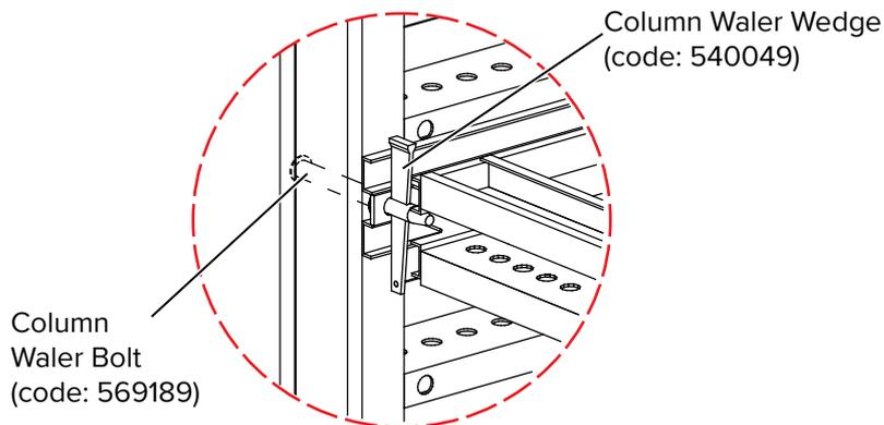
After assembling the panels, the MANTO Column Angle Walers must be mounted. The spacing of the MANTO Column Angle Walers should be adjusted to the desired column dimension by using the captive safety pin.
