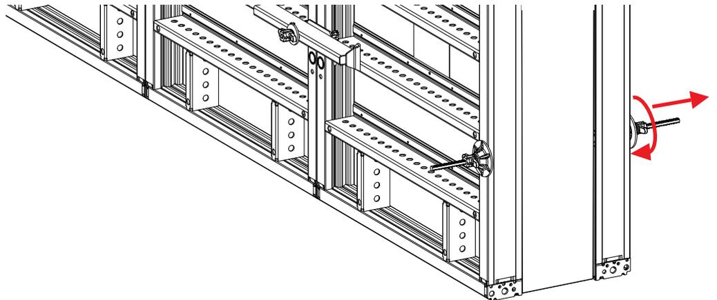
**Step 2** Unscrew the Tie Rod with the Tie Nut from the opposite panel.
