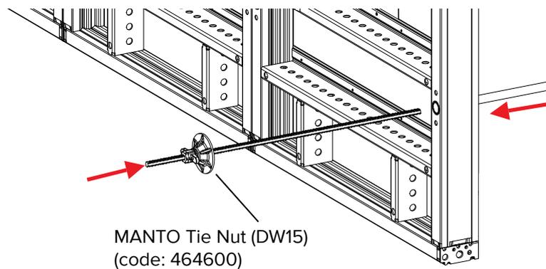
**Step 3** Set up the opposite panel and push the Tie Rod all the way through. Screw the MANTO Tie Nut onto the opposite side of the Tie Rod and tighten by rotating the opposite Tie Nut.
