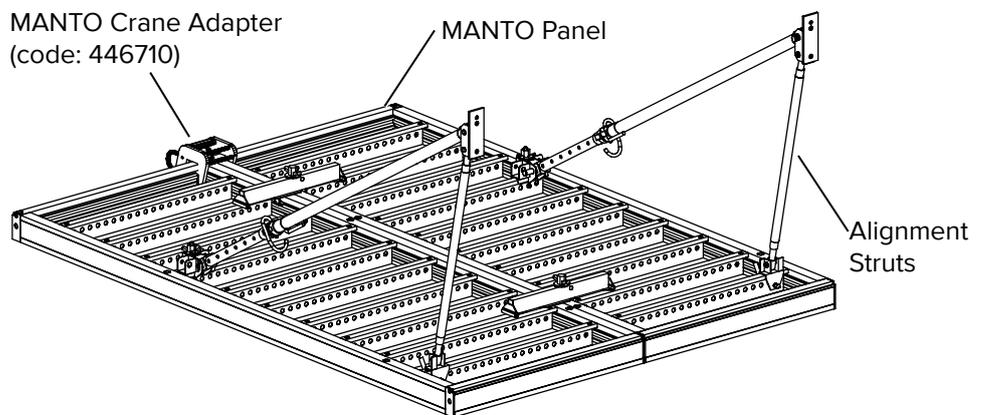
**Step 3** If no pouring platforms are to be attached, the MANTO formwork can now be transported with a crane to the point of use by using the MANTO Crane Adapter.
