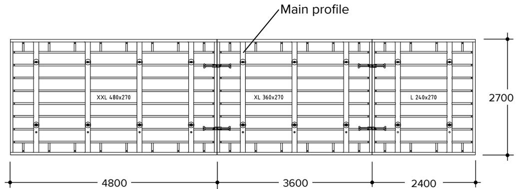
or when used in the horizontal position (main profile is horizontal):
