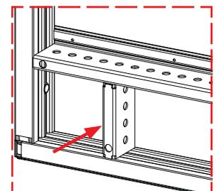
Stiffener elements between ribs and/or between ribs and smaller edge profiles (in most panels).
