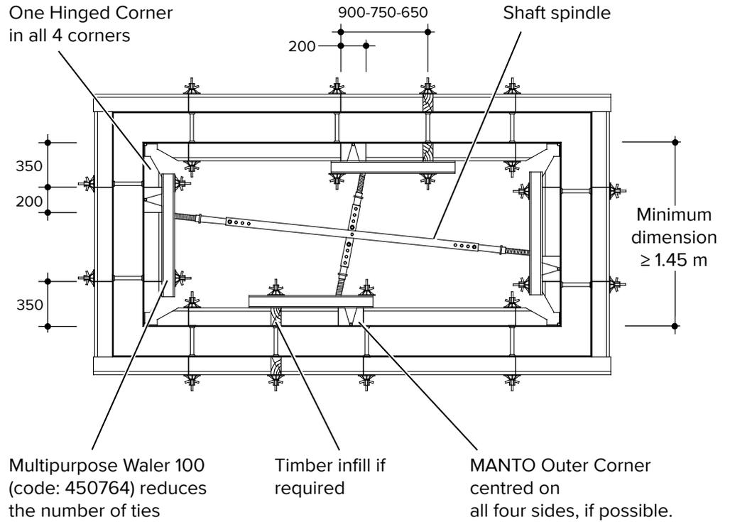
Up to a formwork height of 3.30 m, one shaft spindle is positioned in every direction. Connect the MANTO Outer Corner with a Panel Clamp and an Aligning Panel Clamp to the adjacent panel. The Aligning Panel Clamp serves as a stopper when closing the formwork.
