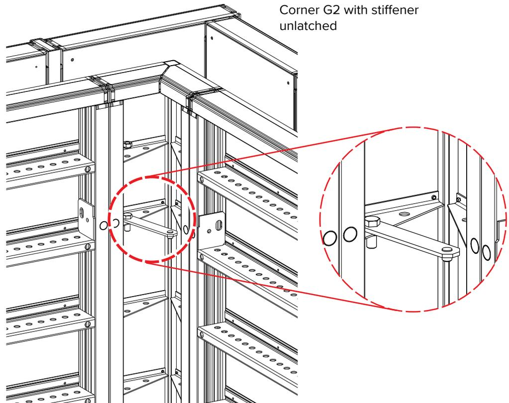
The right-angled outer corner is always made of 2no. MANTO Panels aligned and connected with Outer Corner Clamps. The desired wall thickness can be achieved using the available elements of 300 mm to 900 mm and the MANTO Corner Adjustment.
