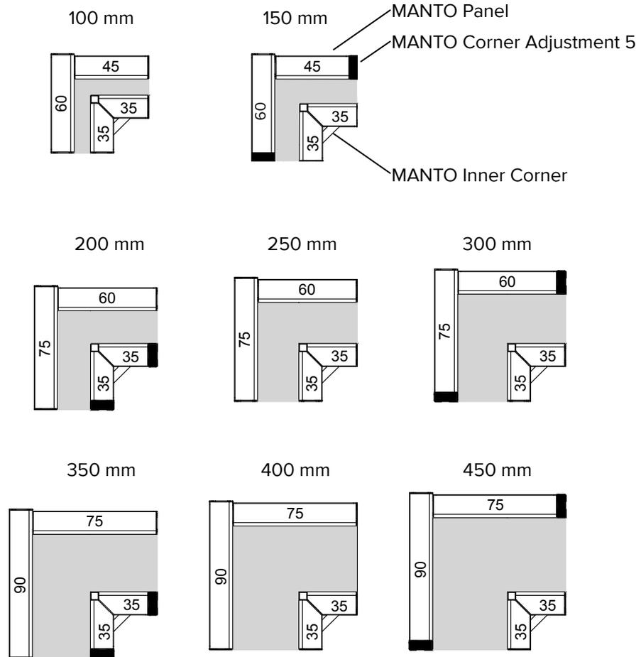
**System dimensions of the typical MANTO corner arrangement**
