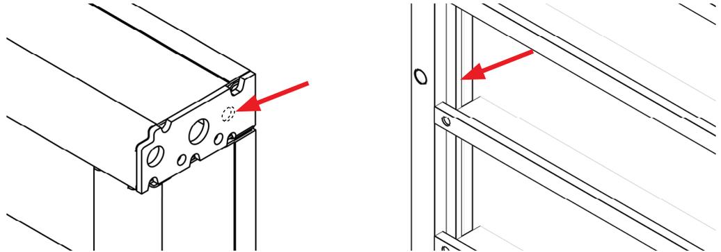
MANTO Panels without  $\varnothing 14$  mm hole in the corner plates and with reinforcement plate on the inside of the long edge profile near the tie positions:
