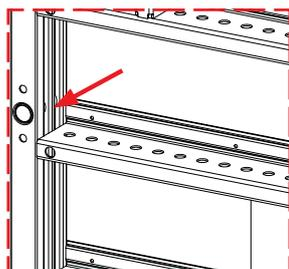
No reinforcement plates on the inside of the long edge profile, near the tie holes.
