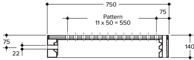
The panels are connected with the MP Bolt, the MP Nut and the Tie Nut 230. For forming heights of up to 2.70 m, only 2no. connections per panel are required.
