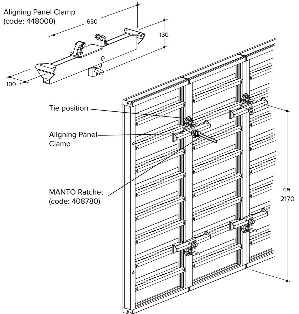
The Aligning Panel Clamps is easy to use for vertical joints when working at ground level (for single-storey formwork).
