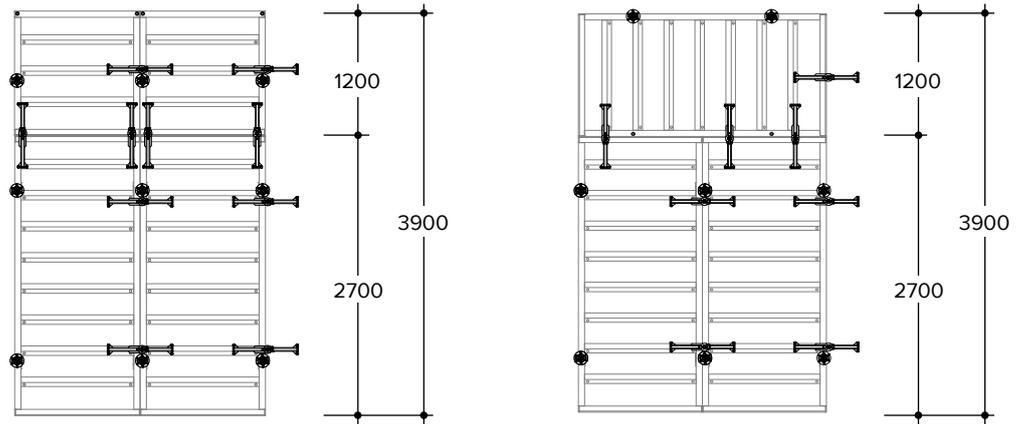
Formwork height: 4.35 m to 4.50 m
