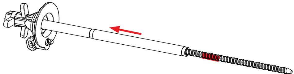
**Step 6** Unscrew the MR Tie Rod until the end of the Tie Rod Sleeve is positioned at the tie rod marking.
