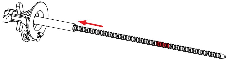
**Step 5** Place the Tie rod Sleeve with the Sealing Cones on the Tie Rod.
