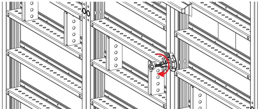
**Step 14** Insert the locking screw of the MANTO G3 Front Tie Nut and tighten.
