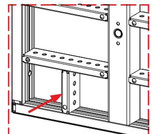
Stiffener elements between ribs and/or between ribs and smaller edge profiles.
