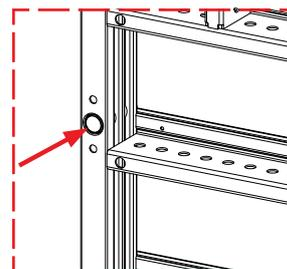
Tie position on the long edge profile with smaller ancillary holes for single-side operated anchors.
