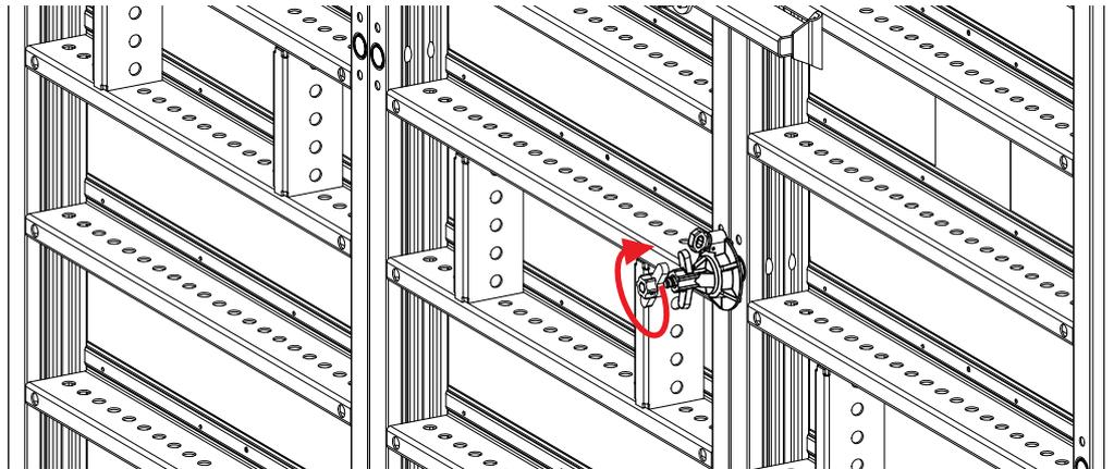
**Step 12** Rotate the washer of the MANTO G3 Front Tie Nut until the locking screw is aligned with the smaller holes in the tie position.
