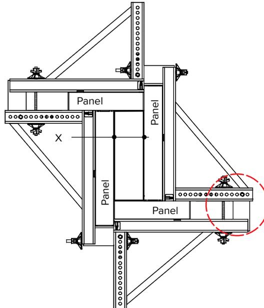
For a column with a cross-section of 350 mm for example, assemble as shown in the details below.
