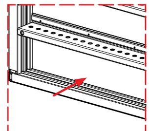
No stiffener elements between ribs and/or between ribs and smaller edge profiles.
