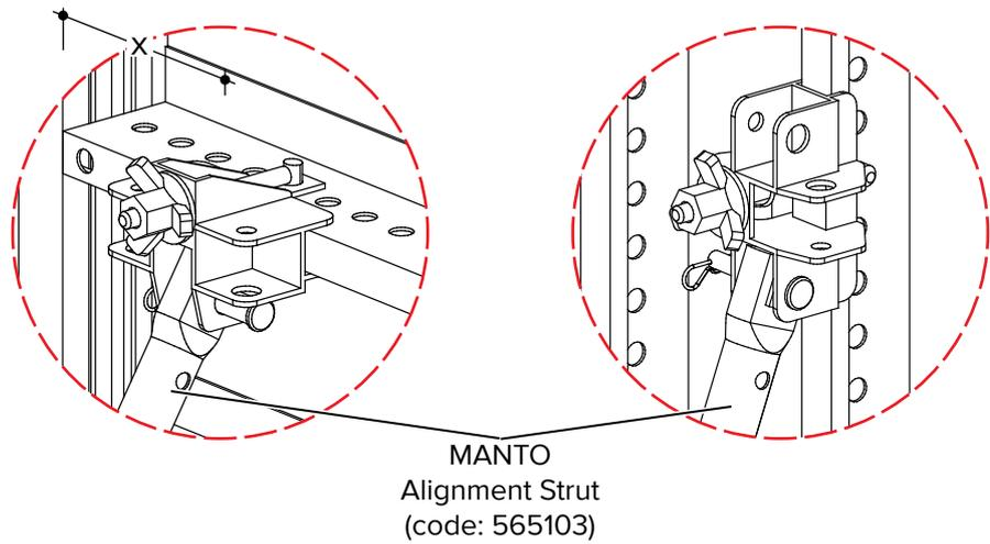
Base connector of the Alignment Strut
