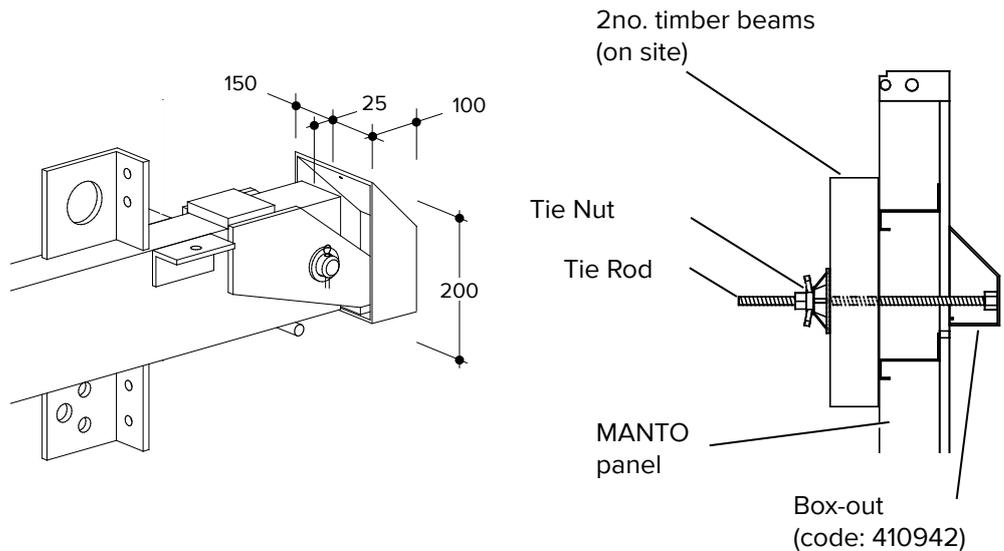
The Box-out can be connected to the MANTO panel with a Tie Rod and a Tie Nut. The Box-out can also be nailed to the formwork using the nailing holes.
