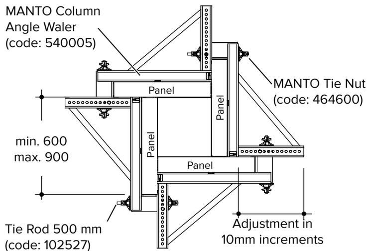
Panels ranging in width from 600 mm to 90 mm can be used to create non-square columns. The marking of the hole pattern allows easy adjustment to the desired column dimensions. Find the hole on the grid with the appropriate dimension and connect it to the hole with the number preceding the dimension (1 to 4).
