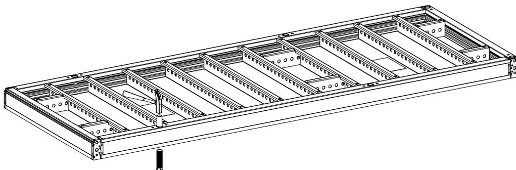
The Punch can also be used to remove concrete residue from the tie holes in the panels.
