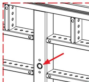
Central profile with tie positions with smaller holes above and below the tie hole for single-side operated anchoring.
