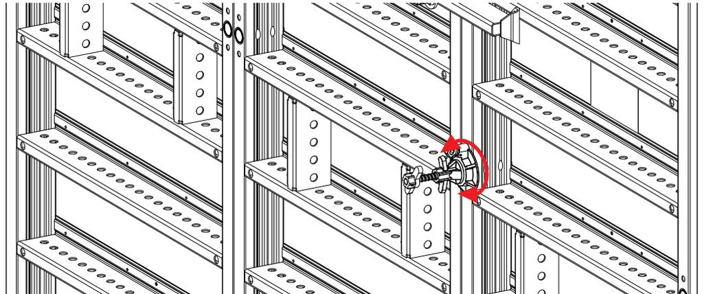
**Step 13** Screw the tie rod wing nut on the MANTO G3 Front Tie Nut as far in as possible.
