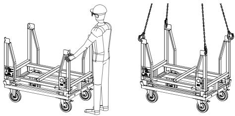
**Step 5** To unload the Euro Stacking Frame, release the four locks in reverse order. Lift the Euro Stacking Frame off of the Euro Trolley
